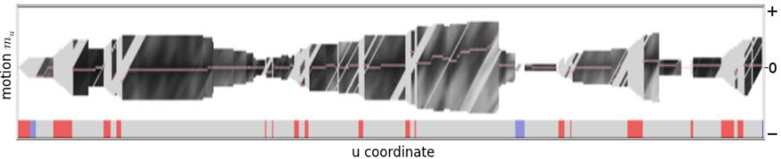
Figure 3: Example motion cost matrix (frame 8). Estimated  $m_u^*$  shown in pink. Red stixels in the lower part correspond to occluded areas in either of the stereo images, blue stixels are the ones assigned to *null motion*, grey stixels are estimated normally.
