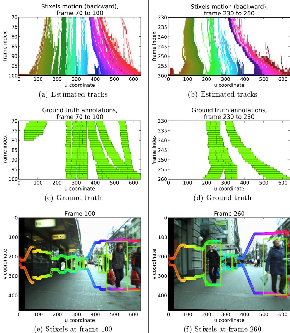
Figure 7: Example of tracks obtained by our algorithm. Sub-figures (a) and (b) show the tracks obtained by backward propagation of the stixels of the latest frame (shown in (e) and (f) respectively). Lighter colours indicate stixels marked as “pedestrian” in the ground truth annotation of the latest frame. Darker colours are other tracked objects (the wall).
