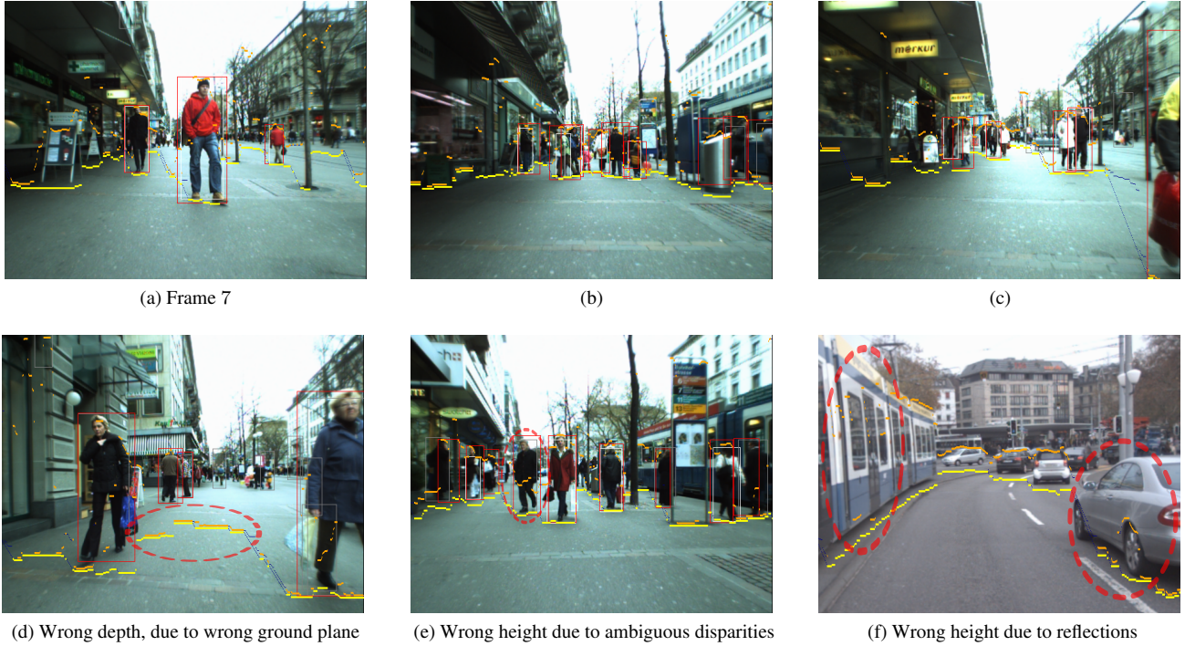
Figure 5: Examples of good results (a,b,c) and failure cases (d,e,f). Red boxes indicate ground truth, the grey boxes the raw results from the detector, and the white boxes the detections validated by the stixels estimate. The lower yellow line and the upper orange line indicate the stixels bottom and top respectively. Dark blue pixels indicate occluded stixels.
